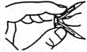
Fig. 18 - Popping Open Anchor Wing For Thin Walls
